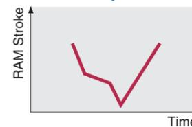
Full control of the ram speed within one punching cycle achieves the ultimate reduction in noise and vibration.
