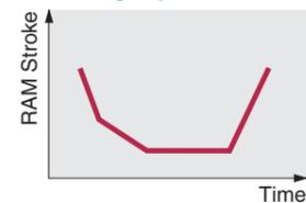
Using variable servo motor control ram stroke between top dead center and bottom dead center, the best results and excellent performance in forming tool operation can be achieved. An important benefit of controlling the ram stroke is to specify a dwell time at bottom dead center and allow material flow during the forming operation.
