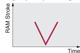
The servo motor is driven alternately between hover height and bottom dead center with a back and forth motion. The hover height position is adjusted based on material type and thickness. This control of the ram stroke provides high speed punching and efficient productivity.
